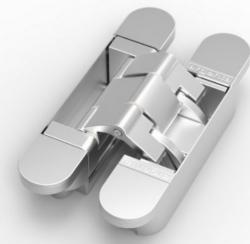
You can adjust these hinges with precision easily, flexibly, and quickly, thanks to the built-in height-adjustment system. This unique system means you no longer need to put any wedges under the door to set the height. The hinge casing is the door can be assembled beforehand in the workshop.
